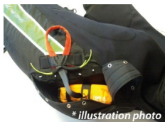
Inserting rescue system into container
